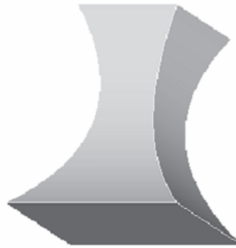
Figure 7-26 Parallel blend with smooth edges
