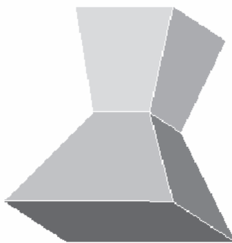
Figure 7-25 Parallel blend with straight edges
